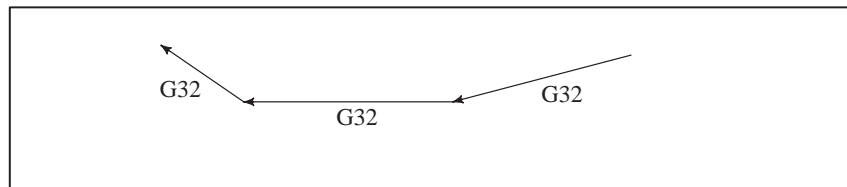
Fig. 4.9 (a) Continuous Thread Cutting
